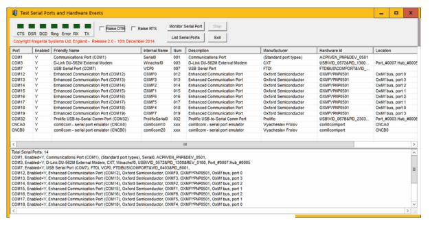
If a modem is connected to the serial port and it has front panel indicators, toggling DTR will cause TR to flash, confirming that the modem is cabled correctly to the PC. If a null modem cable is used to connect two PCs each running the utility, the opposing DSR and CTS indicators will appear as DTR and RTS are toggled on each PC.
