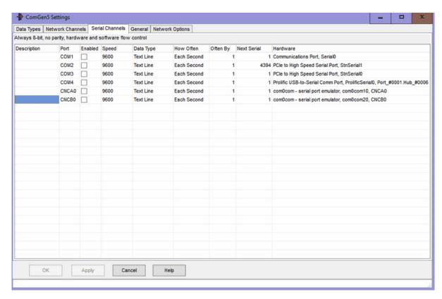
Serial RS232 port configuration is very similar to that in Common Settings, Serial Ports. Note that ComGen only support 8 bit's for data with 1 stop bit and no parity. Some virtual ports may have strange names like CNCA2, but these will work identically to those starting with COM.
