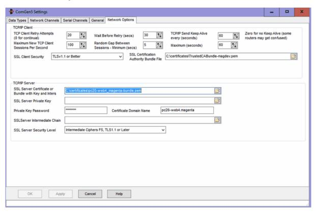
The same SSL certificate will be used for all TCP/IP Server streams. There is no remote server certificate checking for TCP/IP client.
